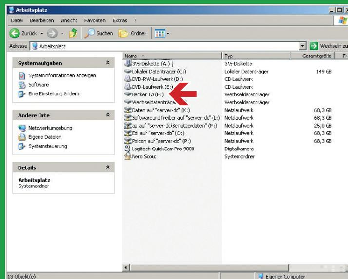
Fig. 1: Recognition as a removable storage device
